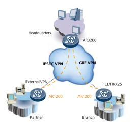
The AR1200 provides various secure access functions to implement communication between enterprise branches and between branches and the headquarters, and to enable partners to access enterprise resources. Tunnels such as GRE VPN and IPSEC VPN are set up between the headquarters and branches to implement secure data access and transmission. The AR1200 implements fast tunnel deployment and authentication for branches. Using a tunnel, partners can access and share enterprise resources.
