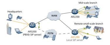
is used as a backup for calls. When the SIP server at the headquarters is unreachable, the built-in local SIP server of the AR1200 implements communication between branches and communication between branch and PSTN network. This ensures reliability of the voice service.
