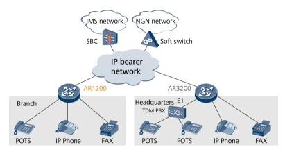
The AR1200 integrates voice, fax, and IP services. When providing voice services for enterprise users, the AR1200 functions as the SIP access gateway of a branch to transform phone signals into VoIP signals. The AR1200 uplink interfaces are connected to the IMS/NGN
