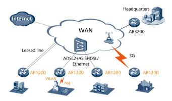
The AR1200s function as the egress routers of enterprise branches and provide flexible access methods to support remote network connections. An AR1200 meets various access requirements, including leased line, Ethernet, xDSL, 3G, and WLAN. This saves deployment and maintenance costs and provides a large value to customers. The fixed 100M Ethernet interfaces of AR1220V, AR1220W and AR1220VW support the PoE function in compliance with IEEE 802.3af
