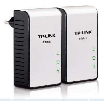
Extend your network via household electrical wiring, no new wires required
