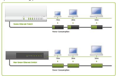
(b) ES-5800G can detect the link status of each port. When the port is idle, the ES-5800G will reduce it's power usage.
