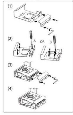
Screw the mounting plate into the desk and make sure it is secured.
